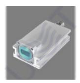
PLL LNB with AGC L.O. 10.6 is professional low noise block down converter with automatic gain control, wide dynamic range of up to 50 dB (biggest among any other LNB). AGC range of 25 dB, LO instability of 50 kHz, Gain (min) of 40 dB.
