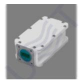
Ku-band LNB PLL with AGC LO 9.75 is low noise block down converter with automatic gain control. It is professional LNB with wide dynamic range – up to 50 dB (biggest among any other LNB). AGC range: 20 dB, LO instability: ± 25 kHz, Gain (min): 34 dB.
