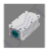
Ku-band LNB PLL with AGC LO 13.05 is low noise block down converter with automatic gain control. It is professional LNB with wide dynamic range – up to 50 dB (biggest among any other LNB). AGC range: 20 dB, LO instability: ±25 kHz, Gain (min): 34 dB.
