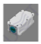
Ku-band LNB PLL with AGC LO 11.80 is low noise block down converter with automatic gain control. It is professional LNB with wide dynamic range – up to 50 dB (biggest among any other LNB). AGC range: 20 dB, LO instability: ±25 kHz, Gain (min): 34 dB.
