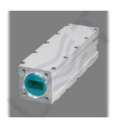
Ku-band LNB PLL dual LO 9.75 10.6 is Low Noise Block Down Converter with dual local oscillator 9.75 GHz and 10.6 GHz and dual 75 Ohm F-type output. LO instability: ± 10 kHz, Gain: 55 dB, Noise figure: 0.8 dB, Output power P1dB: +6 dBm.
