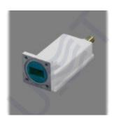
Ku-band LNB DRO LO 8.80 is Low Noise Block Down Converter with single LO 8.80 GHz and single 75 Ohm F-type output. LO instability: ± 2 MHz, Gain: 58 dB, Noise figure: 0.9 dB, Output power P1dB: +3 dBm.
