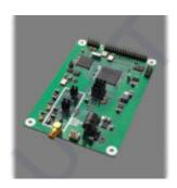
L-band DVB-S-S2-T modulator board is designed for DVB TS (transport stream) modulating, creating the L-band IF signal from parallel TS for further broadcasting in DVB-S, DVB-S2 or DVB-T standards.
