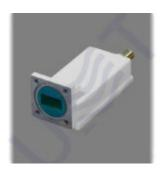
Ku-band LNB DRO LO 11.30 is Low Noise Block Down Converter with single LO 11.30 GHz and single 75 Ohm F-type output. LO instability: ± 2 MHz, Gain: 58 dB, Noise figure: 0.9 dB, Output power P1dB: +3 dBm.
