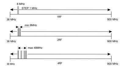
The range of the output frequency adjustment for 3 configuration variants: 1RF, 2RF, 4RF
