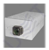
BUC-Ku20-8.8 v2 is block up-converter with fixed output power P1dB **20 W** (ALC power: 2000 mW) and LO of **8.8 GHz**.
