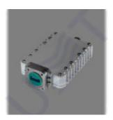
BUC-Ku01-10.6 v2 is block up-converter with fixed output power P1dB **1 W** (ALC power: 100 mW) and LO of **10.6 GHz**.
