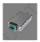
BUC-Ku002-13.05 v2 is block up-converter with fixed output power P1dB **0.2 W** (ALC power: 30 mW) and LO of **13.05GHz**.
